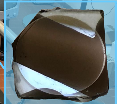
Mg NPs on Pd/glass (SiN x covered)
